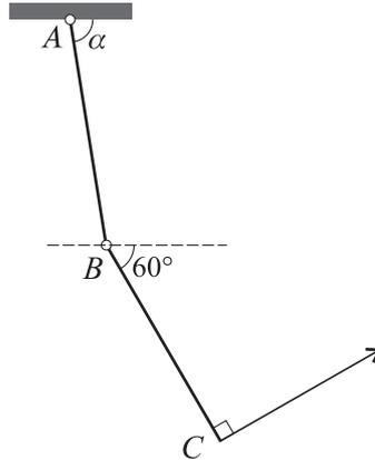
Two uniform rods  $AB$  and  $BC$ , each of length 1.4 m and weight 80 N, are freely jointed to each other at  $B$ , and  $AB$  is freely jointed to a fixed point at  $A$ . They are held in equilibrium with  $AB$  at an angle  $\alpha$  to the horizontal, and  $BC$  at an angle of  $60^\circ$  to the horizontal, by a light string, perpendicular to  $BC$ , attached to  $C$  (see diagram).
